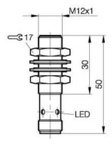
**Inductive Sensors** BES 516-325-G-E5-Y-S 4 M12x1 x 50 normally-open Sn=4mm shielded
